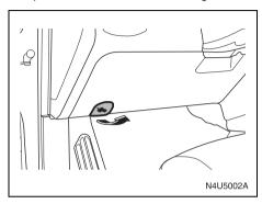
Pull the hood release handle located at the lower left side of the instrument panel.
